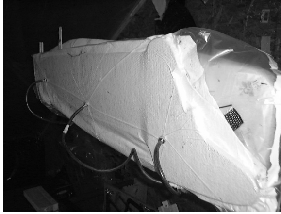
The foil being vacuum bagged.
