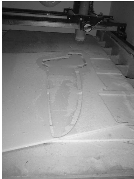
The foil blank (core) shaped out of 5/8" thick 80 kg/m 3 PVC foam (foam saved about 150g compared to western red cedar). The foil is made in two halves, which are epoxied together before over laminating.
