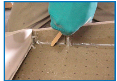
Bottom right: Infusing front bulkhead.
