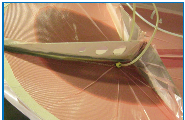
Bottom right: Infusing front bulkhead.
